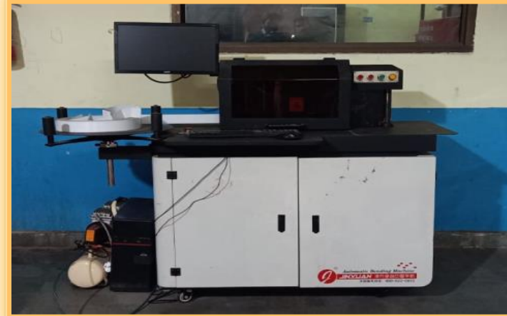
Automatic Chanel Bending Machine
